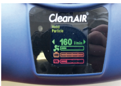
colour display shows the speed of the airflow, the degree of clogged filters and battery charge status
